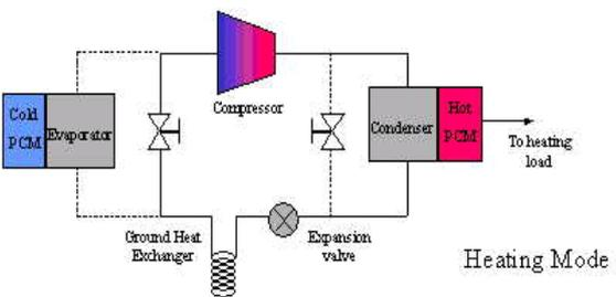
> Using PCM and GHX in heating mode
