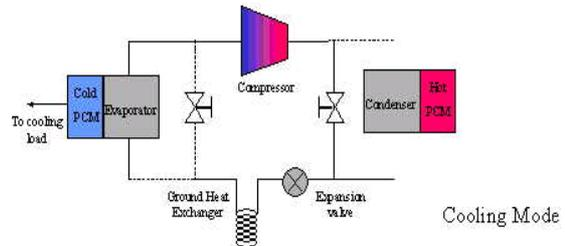
> Using PCM and GHX in cooling mode
