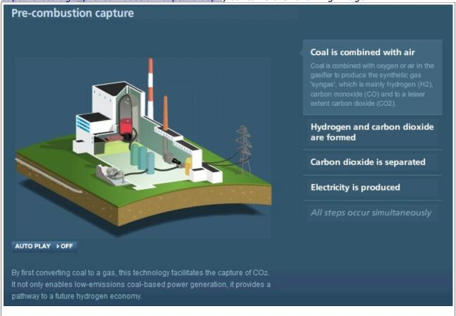
"Syngas" (also known as "water-gas") is, of course, the product of reacting coal with steam - not air or oxygen. The partial combustion of oxygen and coal is to supply the thermal energy needed for the steam/coal reaction which is endothermic. If air is used instead of oxygen for this combustion then the CO2 capture is made more complicated by the need to deal with the dilution of the CO2 caused by adding large quantities of atmospheric nitrogen.
